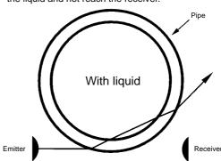
If the diameter of the pipe is close to 6 mm, some of the emitted beam may reach the receiver because the angle of refraction is small, thus making the stable operation of the EE-SPX613 difficult. In such cases, set the sensitivity selector to Low and check that the EE-SPX613 will be in stable operation.
